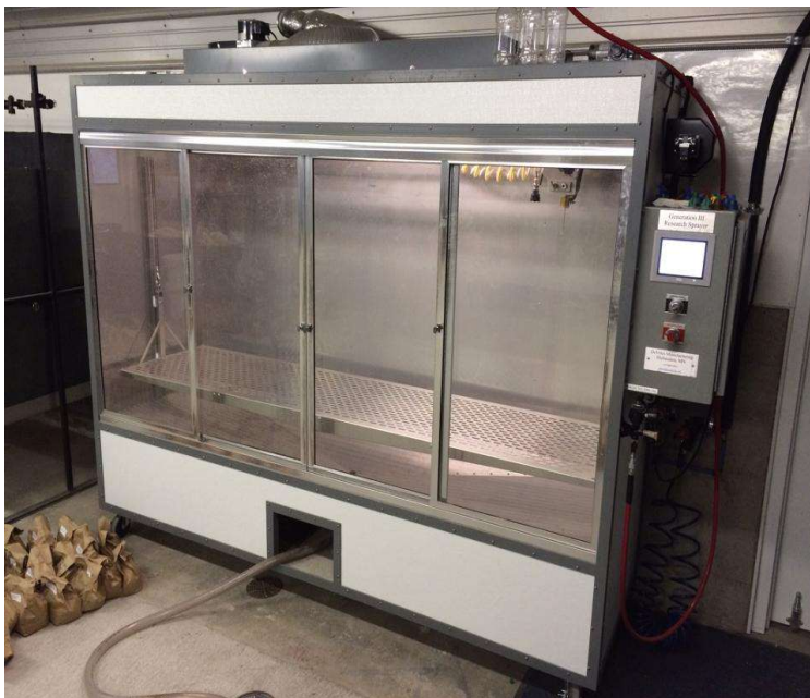
Figure 2. Single nozzle spray chamber located at the PAT lab used to simulate rainfall.
