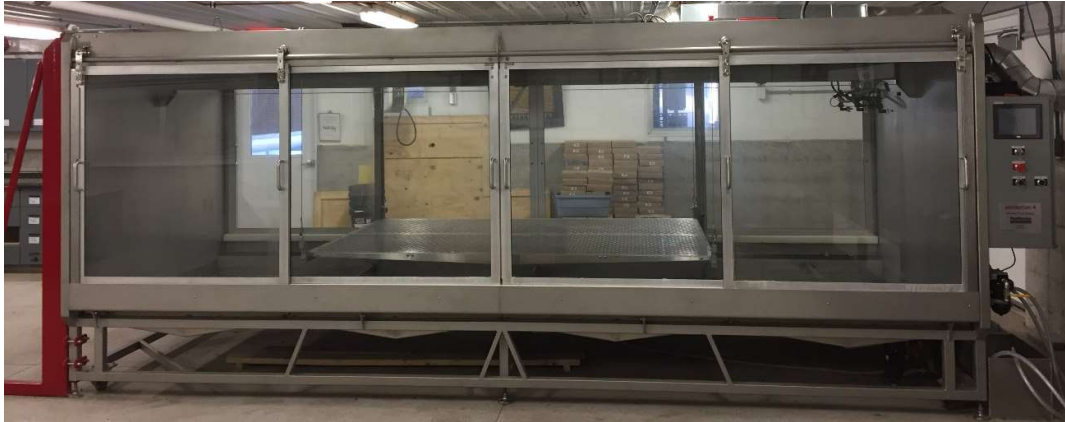
Figure 1. Three nozzle spray chamber located at the PAT lab used to apply treatments.
